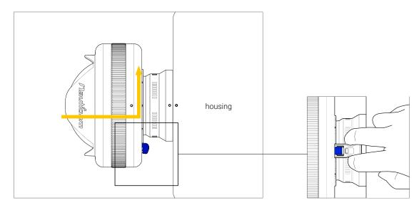
Alternatively, the release extension can be attached onto the lens mount release button on the M67 to bayonet convertor for better ergonomics
